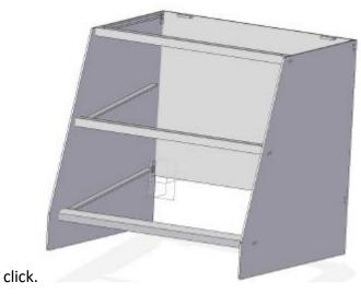
**Step 6**: attach the top cover and use the 4 3/32 screws to attach it
