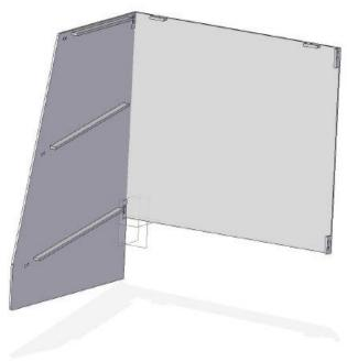
**STEP 2:** attach the right side to the back using the big 18-8 barrels and screws need 4 for this step.
