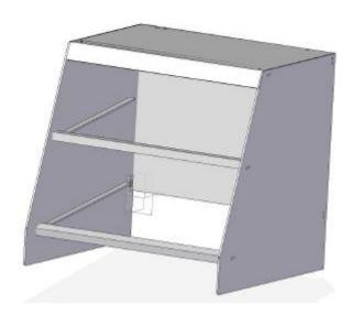
**Step 7:** you can slide the 2 shelves, the smaller one on the top. And you plug the electrical plug on the back of the unit NEVER CLEAN THE UNIT WITH ALCOHOL, WINDEX OR AMONIAC. Clean only with soap and water.
